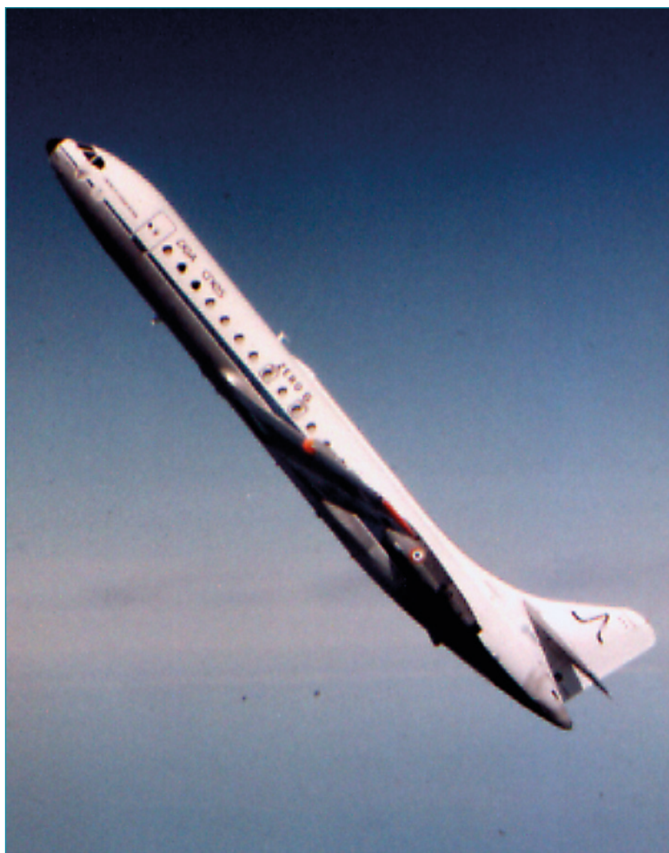
Figure 1. Parabolic flight in a Caravel in France in 1991, during which we measured central venous pressure invasively in eight subjects during short periods (20 s) of weightlessness (Videbaek and Norsk, 1997). The aircraft followed a Keplerian trajectory, whereby a free-fall condition (0 G) was created symmetrically around the top. The 0 G phase was preceded by 20 seconds of pulling up to 2 G and then again followed by an up to 2 G descending phase of similar duration.
