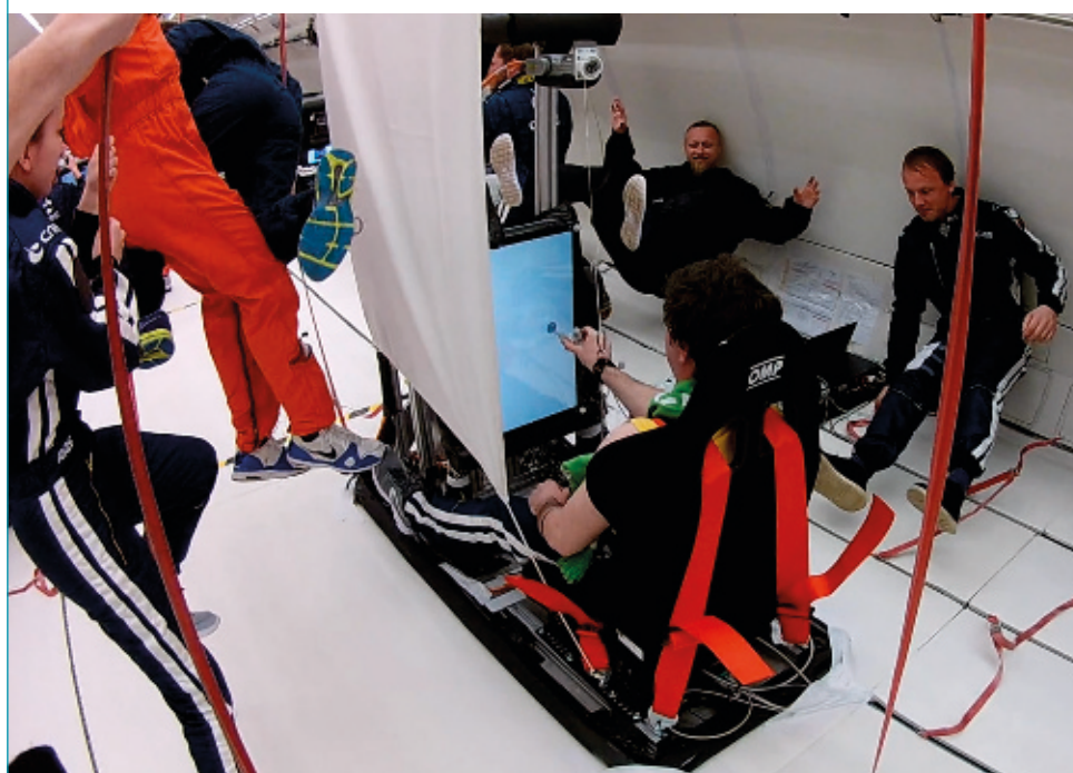
Figure 1. Studies during parabolic flight manoeuvres. The upper panel shows the flight pattern of the Airbus during one parabola (photo: ESA). The zenith of the parabola offers 20 seconds of microgravity. The lower panel depicts human motor-control experiments in zero-gravity environment investigating how the brain encodes gravity and how we can prepare astronauts for the challenging environment during and after space flight (photo courtesy ESA). Principal investigator: Jan Babič, Jozef Stefan Institute, Slovenia.
