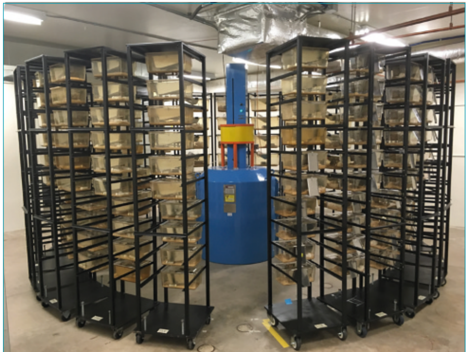
Figure 2. The neutron irradiation facility at CSU. Shown are the annular arrangement of rodent cages around the lead-shielded ^{252}\text{Cf} source that can be lowered and raised for maintenance and animal husbandry procedures. The arrangement of the cages can be modified to accommodate a variety of samples and configurations, and depending on the actual distance from the source, dose rates can be adjusted accordingly.
