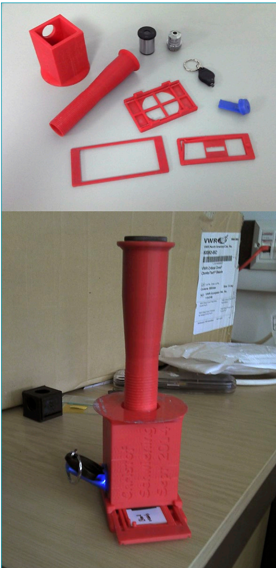
Figure 7. With a spare objective, an eyepiece, a cheap LED and some 3D printed parts (left) it is possible to make a fluorescence microscope (middle) capable of showing live Zebrafish encoding GFP (right). Once assembled and with the Zebrafish in position, the microscope is pushed down clamping the stage in place allowing the microscope to be passed between a group of A level students. (Christof Schwiening, PDN).
