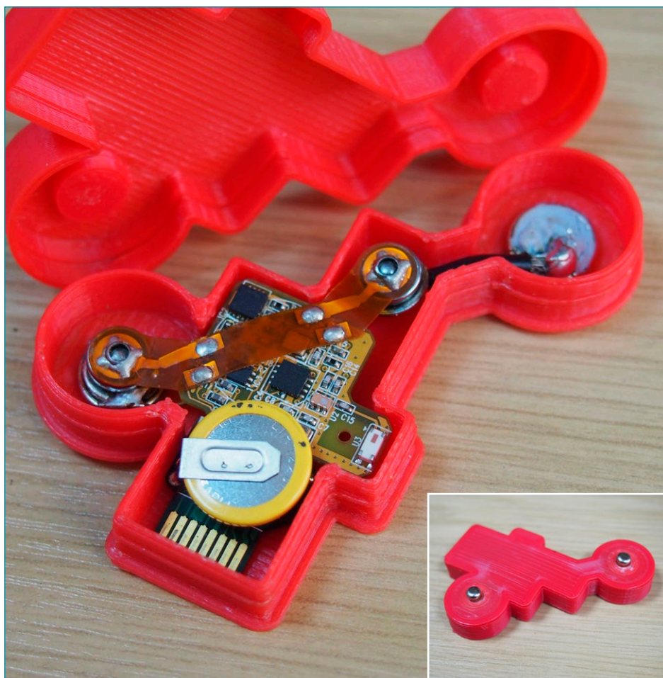
Figure 5. Making cheap electronics robust without adding weight. (Inset) An OPI TrueSense Exploration Kit (512 Hz 13-bit A/D, 3 axis accelerometer, temperature sensor, Wifi broadcast and 11+ hours on board recording – £30) mounted in a 3D printed water-resistance case (shown assembled in main picture) designed to clip to a Garmin heart rate strap for ECG recording in a 3rd year BSc project on stair climbing (Christof Schwiening).
