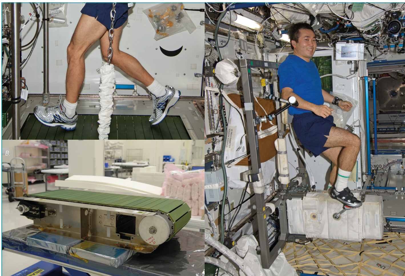
Figure 2. ISS Exercise equipment. A. COLBERT in use on the ISS, B. COLBERT treadmill unit in detail, C. CEVIS in use on the ISS. Images © NASA
