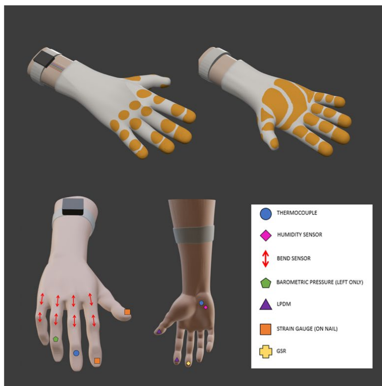
Figure 1: CAD mock-up of sensor placement within PerformGlove. LPDM = Laser Doppler Perfusion Monitor. GSR = Galvanic Skin Response.
